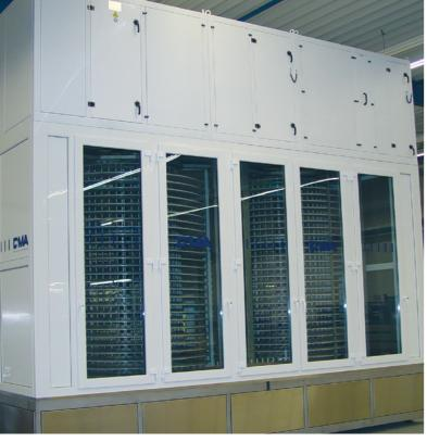
The cooling equipment can be placed in front of, between or above the spirals depending on the available space.
