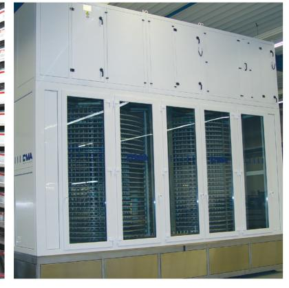
The cooling equipment can be placed in front of, between or above the spirals depending on the available space.
